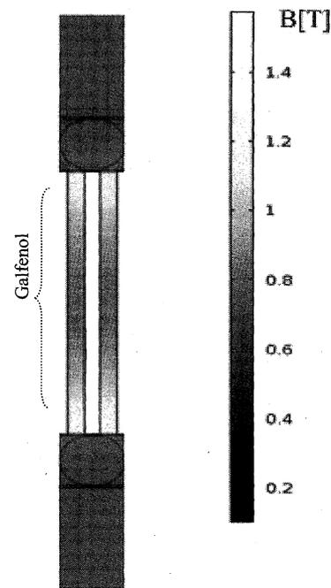
Fig. 6. Magnetic flux density  $B_x$  distribution in a cut view through Galfenol beams without bending load.
