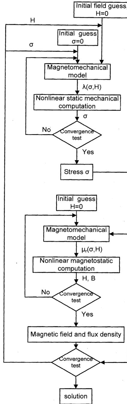
Fig. 3. Diagram of the weak coupling approach.
