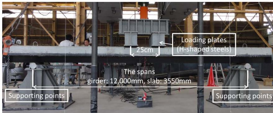
Photograph 1. Experimental equipment for static loading tests.
