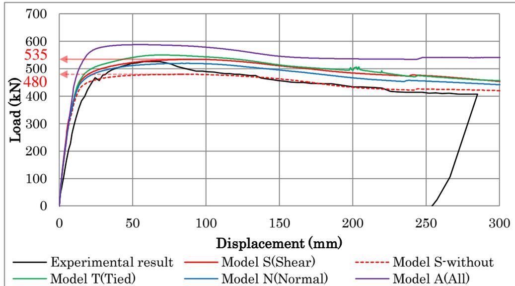
Figure 6. The load-displacement relation of the testing slab.
