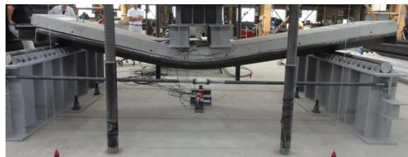
Photograph 3. A static loading test (slab).
