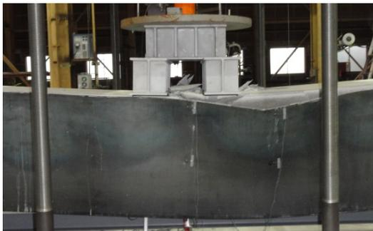
Photograph 2. A static loading test (girder).
