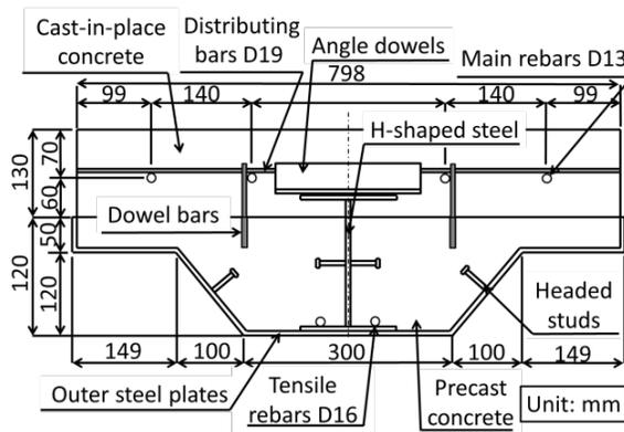
Figure 2. A cross-sectional view of the slab.
