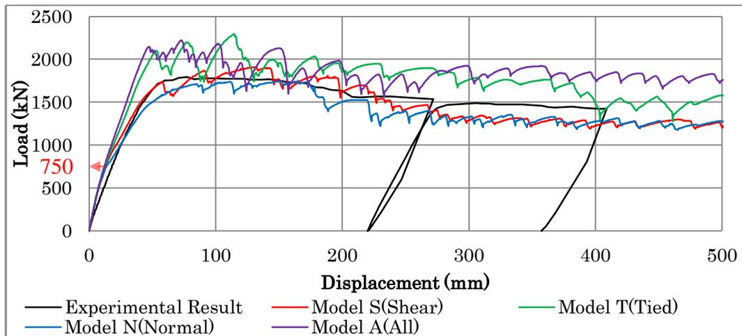
Figure 5. The load-displacement relation of the testing girder.
