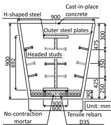
Figure 1. A cross-sectional view of the girder.
