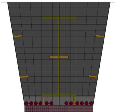
Figure 3. A cross-sectional view of an analytical model of the girder.
