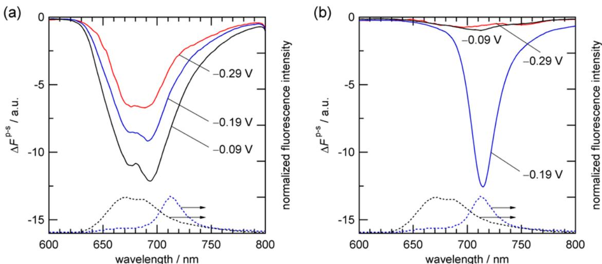
**Figure 3.** PM-TIRF spectra for  $\text{H}_4\text{TPPS}^{2-}$  at the water|DCE interface under the excitation at (a) 404 nm and (b) 488 nm. The pH of the aqueous phase was pH 2.2. The blue and black dotted lines refer to the normalized fluorescence spectra of J-aggregates at pH 1.3 and monomers at pH 2.3 in the aqueous solutions under the excitation at 488 nm.
