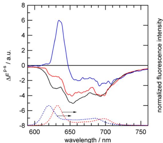
**Figure 7.** The dependence of PM-TIRF spectra at  $\Delta^w\phi = -0.16$  V on the  $\text{H}_2\text{PP}^{2-}$  concentration. The concentrations of  $\text{H}_2\text{PP}^{2-}$  were  $2.0 \times 10^{-5}$  (black),  $1.0 \times 10^{-4}$  (red) and  $5.0 \times 10^{-4}$  mol  $\text{dm}^{-3}$  (blue). The blue and red dotted lines refer to normalized fluorescence spectra measured in the aqueous and organic solutions.
