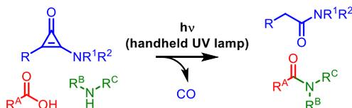
**ABSTRACT:** A phototriggered dehydration condensation using an aminocyclopropenone has been developed. The UV irradiation of an aminocyclopropenone generated a highly reactive ynamine *in situ*, and the dehydration condensation of a carboxylic acid and an amine coexisting in the reaction solution smoothly proceeded to afford an amide. This reaction is completely controllable by the ON/OFF states of a UV lamp.
