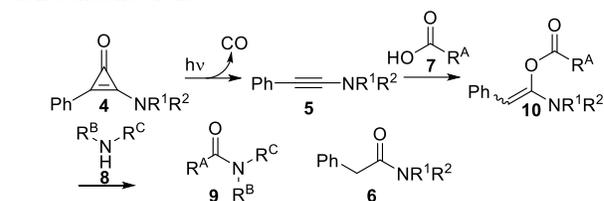
For **4a** and **4c**, a small amount of **9aa** was formed even under dark conditions (**Table 2**, entries 1 and 3). The background reaction in these conditions did not yield the hydrated ynamine **6**, which should be observed if the ynamine **5** would be involved in **9aa** formation. Therefore, the background reaction would occur with a mechanism different from that of the phototriggered dehydration condensation.<sup>18</sup>
