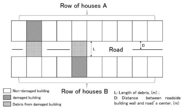
Figure 5 Road blockade caused by debris from a damaged building along a road
