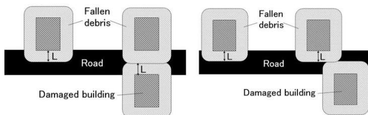
Figure 7. An example of road blockade detection by using the buffer function. The buffer zone was created based on debris length of damaged buildings.
