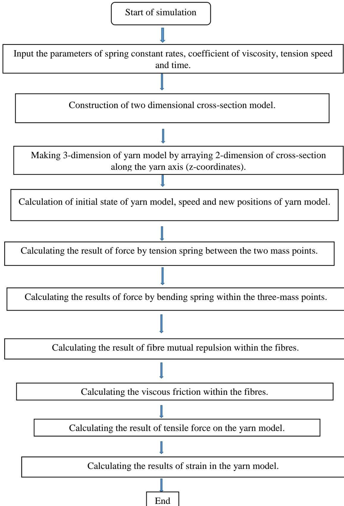
Figure 2.12. Flow chart of simulation aspects for yarn model.
