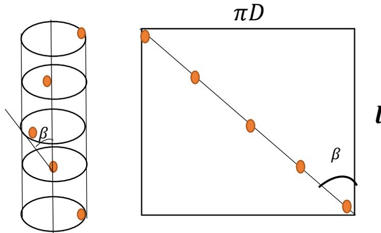
Figure 2.3. Twist angle in the idealised helical yarn structure.
