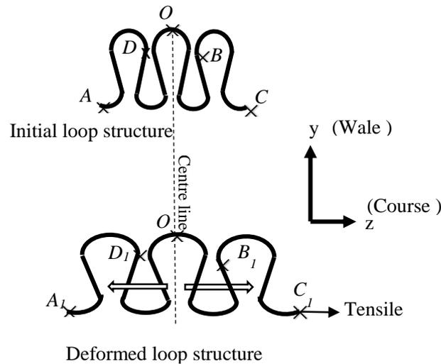
Figure 3.4. Deformation of loop structure pulling in the course direction.
