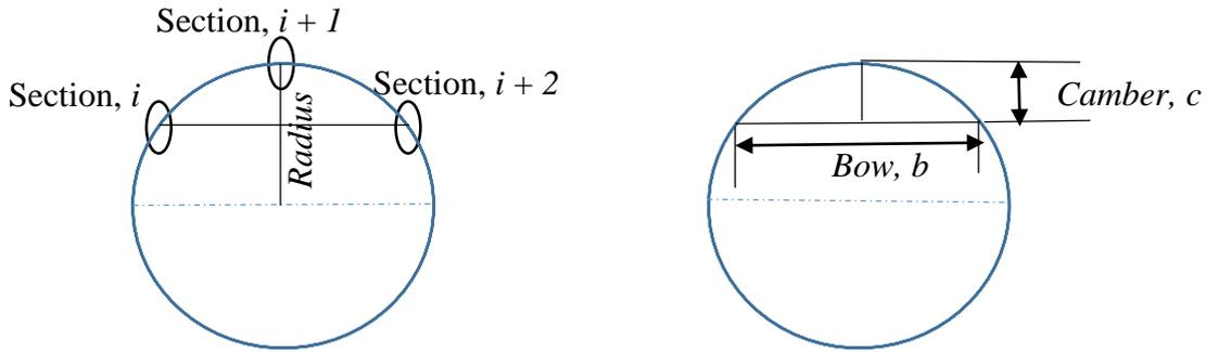
Figure 3.11. Dimensions of cam and bow system used in determination of curvature of each section.
