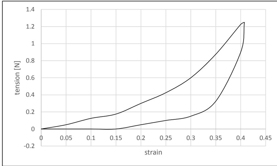
Figure 5.3. Force-strain curve of the sample by KES system.
