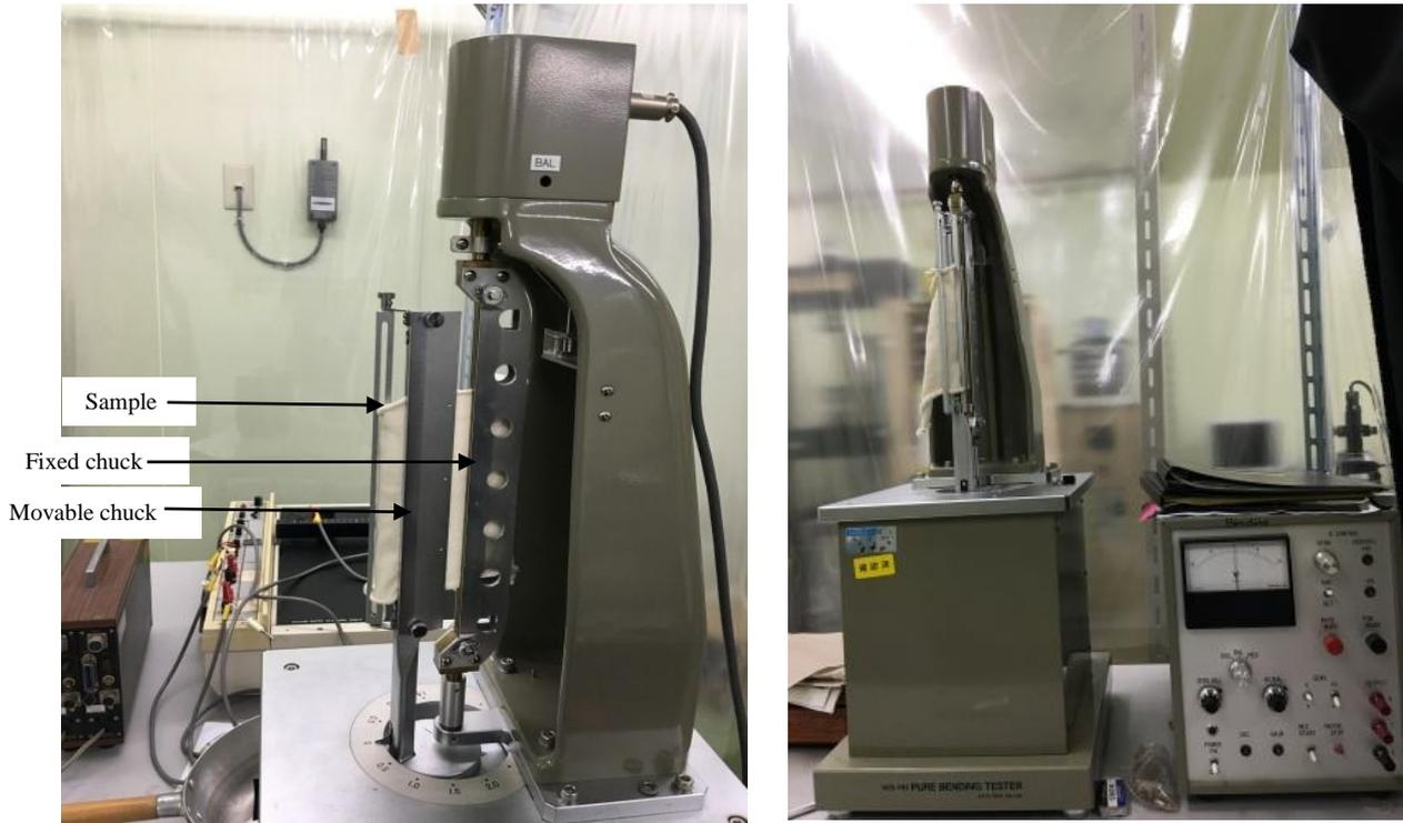
Figure 4.4. Pure bending tester of KES-F2.
