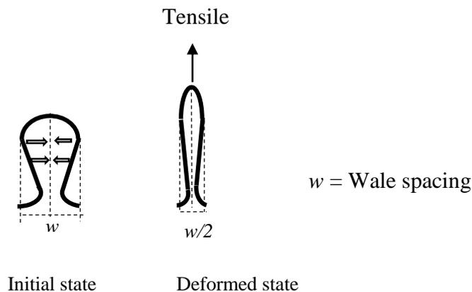
Figure 3.7. Compression of loop structure under tensile in the wale direction.
