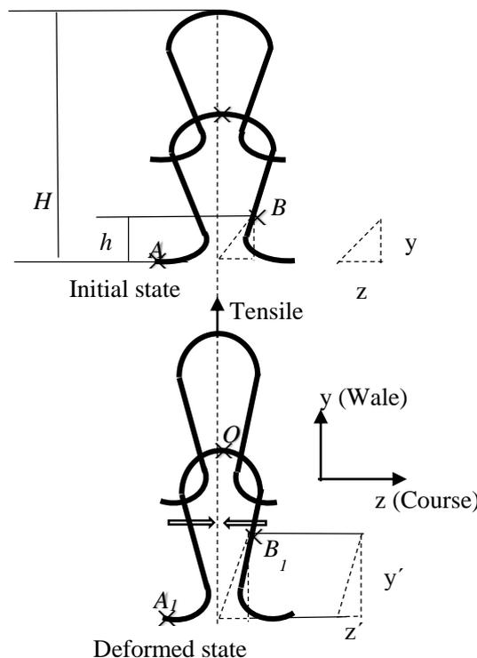
Figure 3.9. Deformation of loop structure under tensile in the wale direction.
