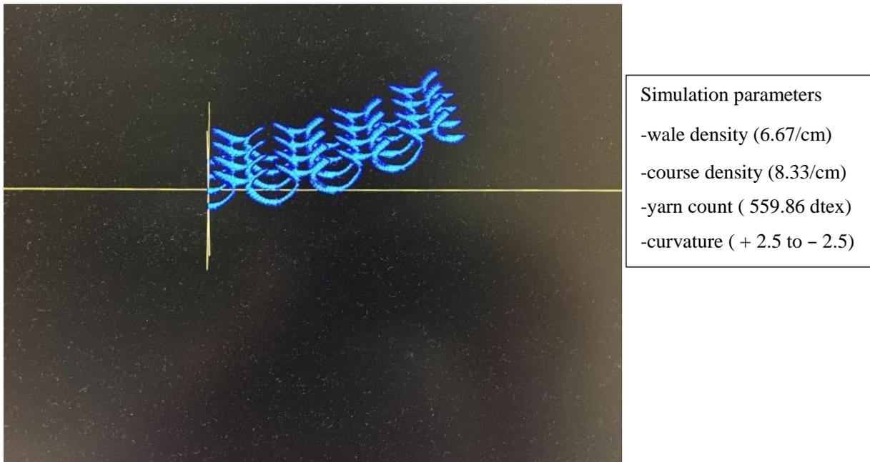
Figure 4.7. Image of course-bending simulation of loop model.
