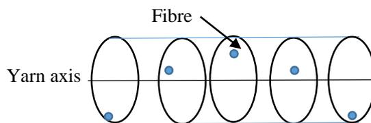
Figure 2.1. Different positions of fibres in the idealised geometric yarn structure.
