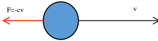
Figure 2.8. Friction force in the mass point.
