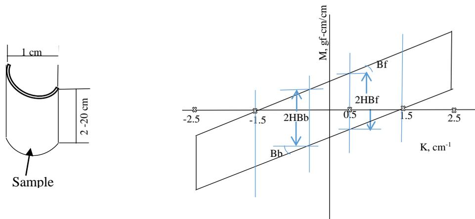
Figure 4.5. Bending property of KES system.
