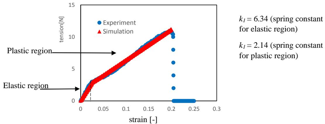
Figure 2.11. Results of simulated yarn model and experimental yarn in tensile properties.
