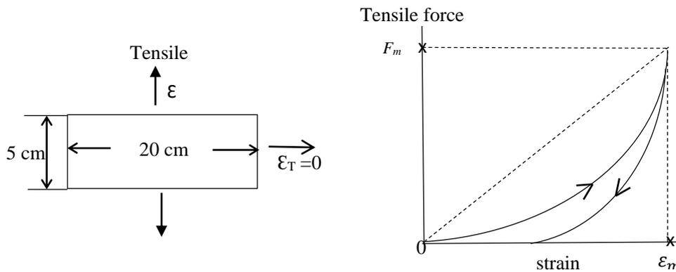
Figure 5.1. Tensile test in KES system.
