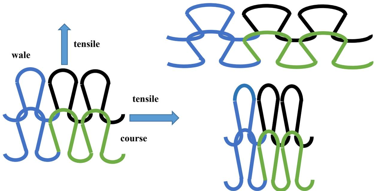
Figure 3.1. Deformation of plain weft-knitted fabric.
