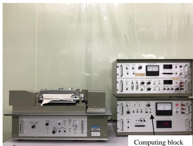
Figure 5.2. Tensile tester of KES-F-1.
