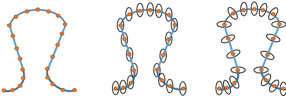
(a) Loop structure with coordinates of centre mass points. (b) Loop structure with cross sections. (c) Loop structure with inclined cross sections.
