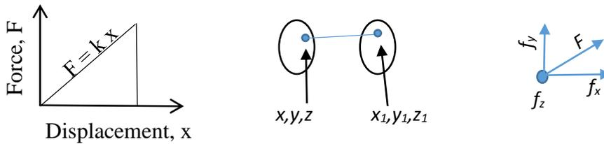
Figure 2.9. General description of force acting on the mass point.
