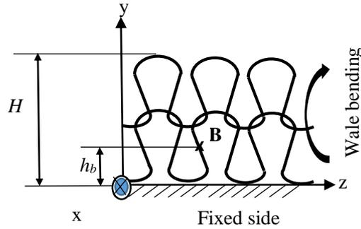
Figure 4.3. The required lengths for the determination of curvature in bending the loop model.
