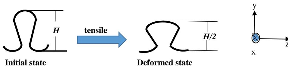
Figure 3.2. Deformation of loop structure according to its course spacing.
