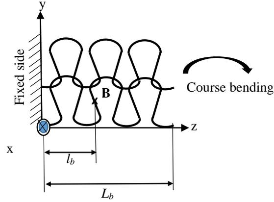
Figure 4.2. The required lengths for the determination of curvature in bending the loop model.
