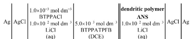
**Figure 1.** Composition of the electrochemical cell.
