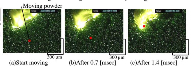
Fig.7 Position of metal powder
