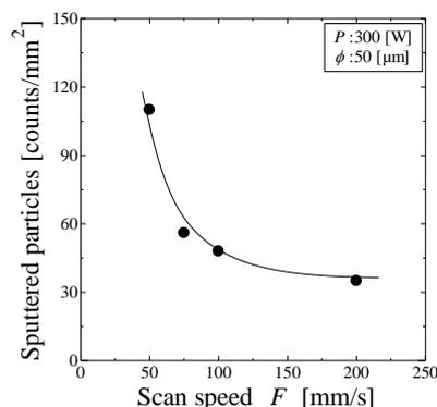
Fig.5 Variation of sputtered particles with scan speed
