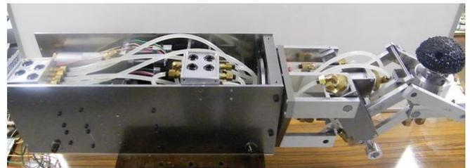
Fig7. Prototype of sewage robot
