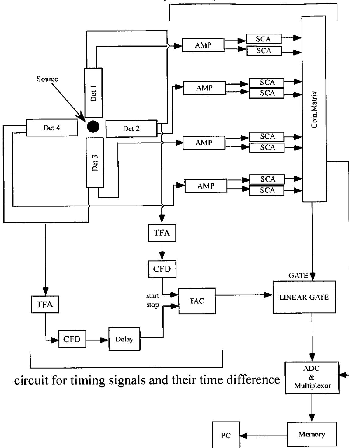
Fig. 2-6 Diagram of electronic circuit for PAC measurement
