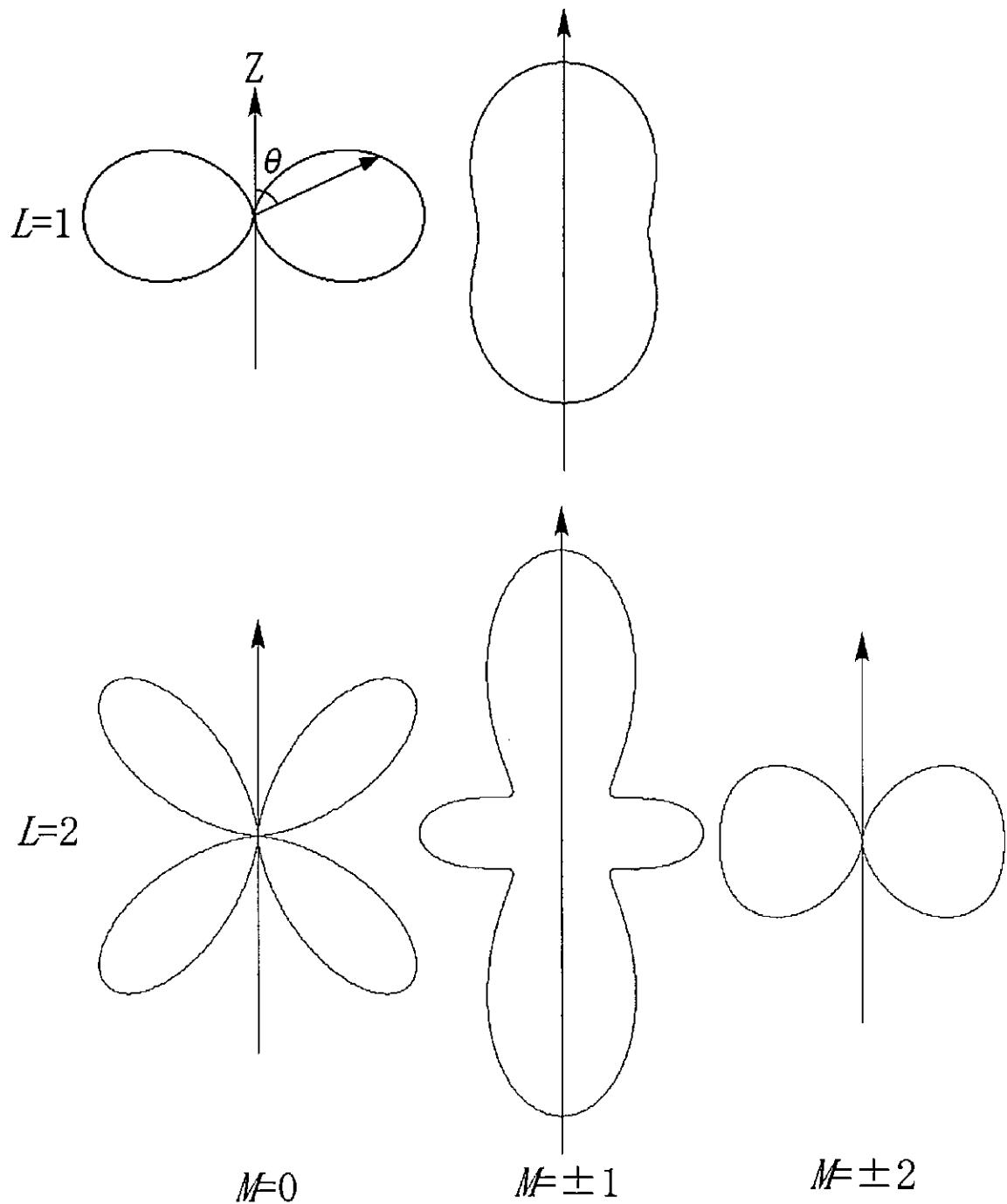
Fig. 1-2 Angular correlation of  $\gamma$ -rays
