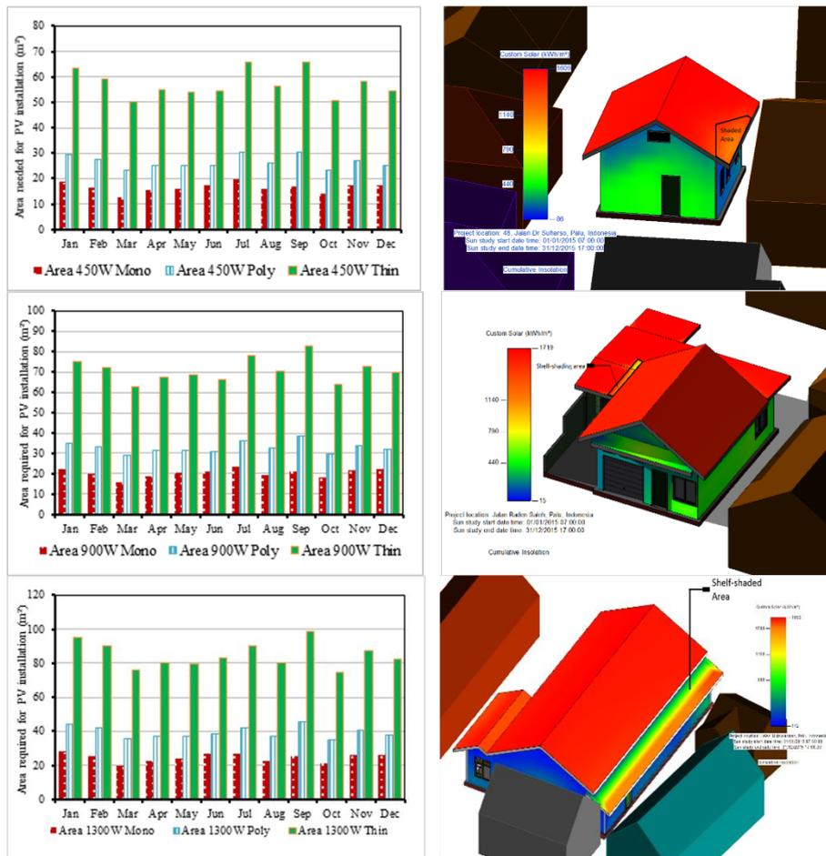
Figure 3.1 Required Area for Photovoltaic Installation on 450W, 900W, and 1300W Model (left) and Annual Insolation Mapped on Building Envelope (right)
