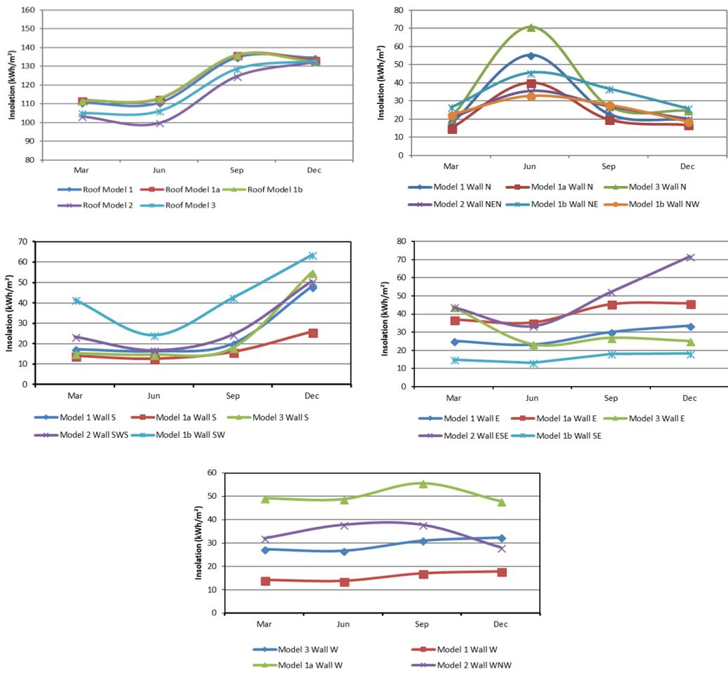
Figure 4.1 Insolation Gain by Building Envelope
