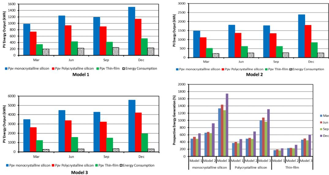
Figure 4.2 Photovoltaic Electrical Energy Generation by the three Models and their Prospective of photovoltaic Installation
