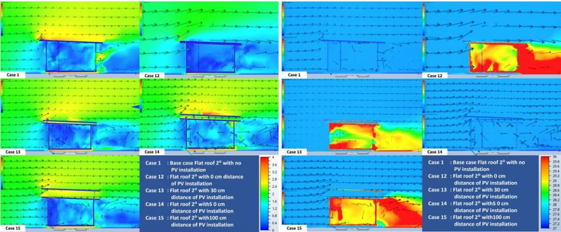
Figure 5.2 Air Velocity in m/s (left) Mean Radiant Temperature in °C (right) Inside and Around the Tested Models
