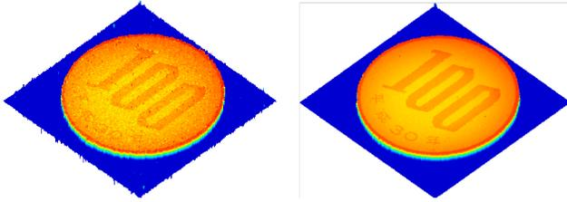
(a) When a DFB laser is used. (b) When a VCSEL is used.
