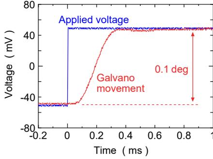
Fig. 14. Step response of the galvano mirror.
