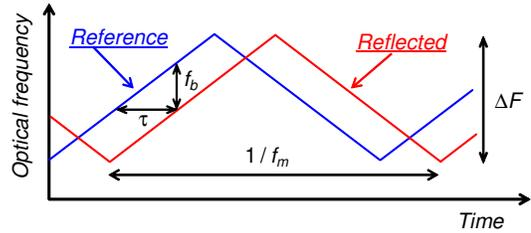
(b) Waveform of optical frequency change.
