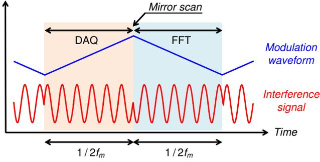
Fig. 10. Timings of the data acquisition (DAQ), the galvano mirror scan, and the FFT analysis.
