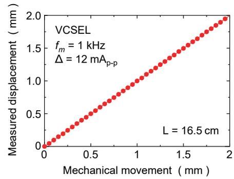
Fig. 8. Measured displacement against the small displacement.
