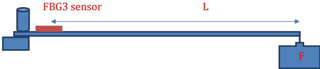
Figure 54. Strain measurement by using the cantilever beam method.
