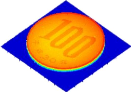
Figure 4.23 Three-dimensional profiling result of a Japanese 100YEN coin using the asymmetric method with  $f_m = 1.0 \text{ kHz}$ ,  $T_r = 620 \mu\text{s}$ ,  $T_f = 380 \mu\text{s}$  and the number of acquired data is 1650 points.
