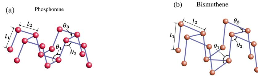
**Fig. 2.** Geometries of (a) phosphorene and (b) bismuthene.
