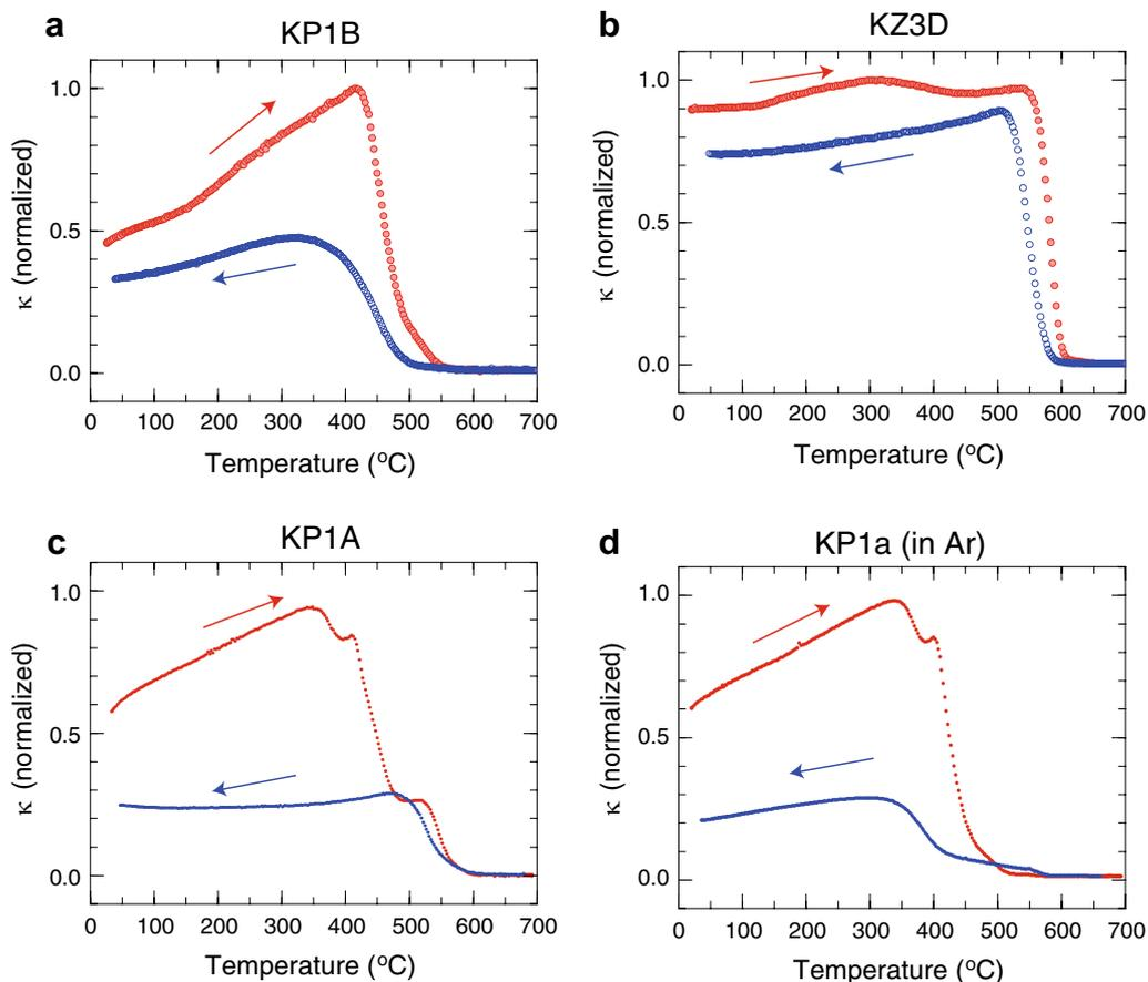
**Fig. 4** Thermomagnetic curves of magnetic susceptibility. Red filled symbols represent heating, and blue open symbols represent cooling. Rock magnetic data. **a** Sample with single Curie point, heating in air. **b** Sample with a Curie point suggestive of magnetite with near-reversible curves, heating in air. **c** Sample with three Curie points, heating in air. **d** Same sample as (c) heated in Ar showing two Curie points
