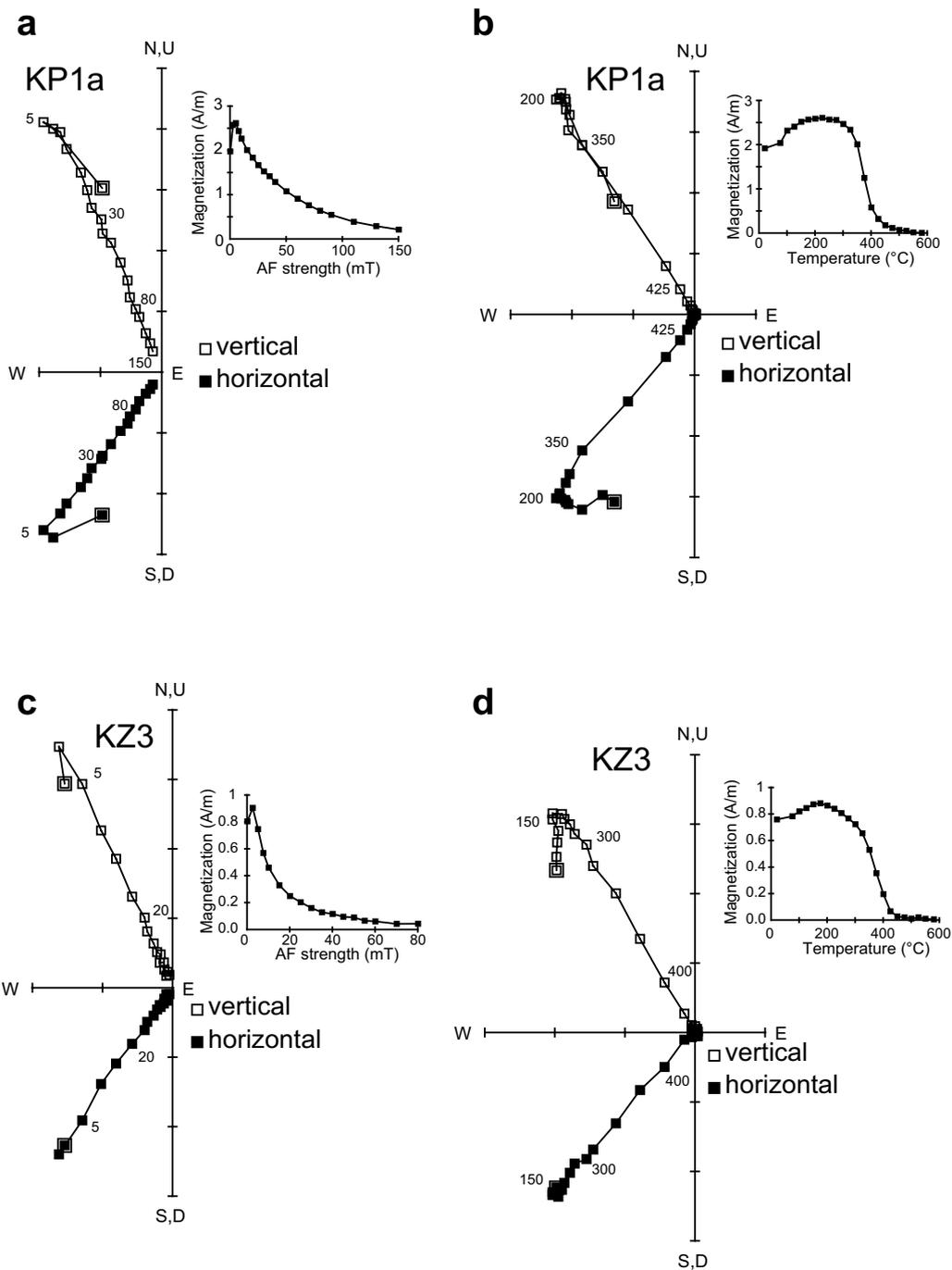
**Fig. 6** Representative demagnetization behavior of tilt-corrected paleomagnetic directions in orthogonal vector plots and magnetization versus demagnetization step plots. **a** AF demagnetization of the sample KP1a. **b** Thermal demagnetization of the sample KP1a. **c** AF demagnetization of the sample KZ3. **d** Thermal demagnetization of the sample KZ3
