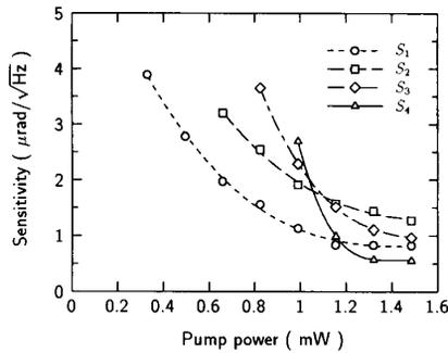
Fig. 4. Measured sensitivities of the sensors against the pump power.
