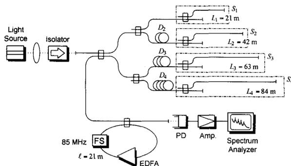
Fig. 1. Experimental setup of a sensitivity enhanced coherence-multiplexed sensor system using an optical loop with a frequency shifter.
