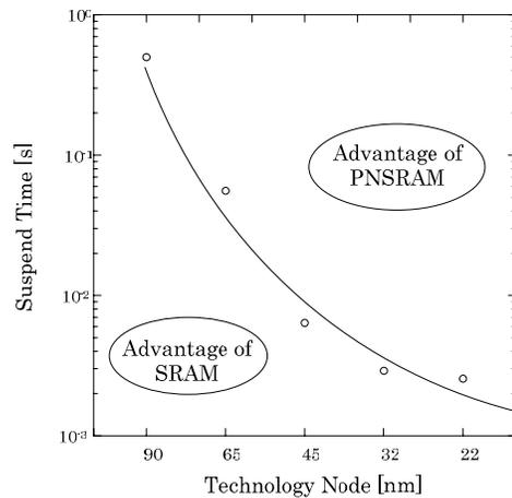
Figure 9. Standby energy comparisons between SRAM and PNSRAM.
