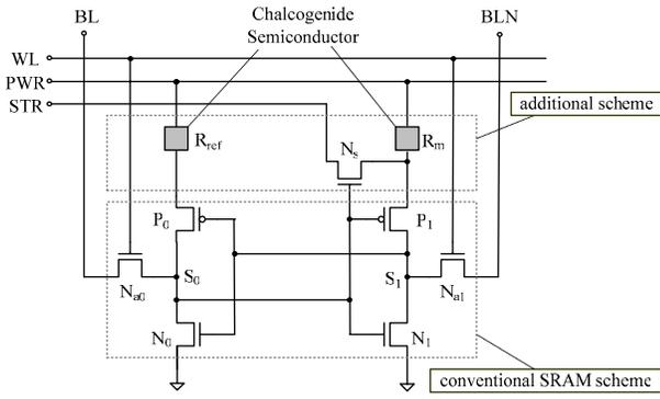
Figure 1. PNSRAM cell configuration.
