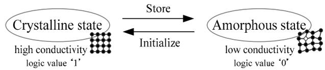
Figure 2. State transition diagram of chalcogenide semiconductor.
