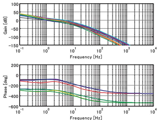
Fig. 8 Frequency response of GK with LSDP controller
