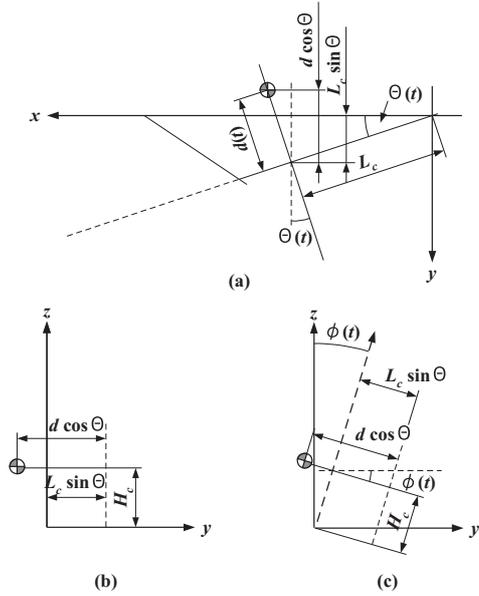
Fig. 5 Center-of-gravity coordinates of a cart
