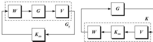
Fig. 6 The loop shaping design procedure
