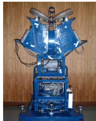
Fig.4 New pitching machine (3 rollers type)
