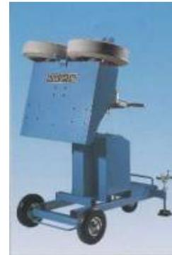
Fig.2 Pitching machine (2 rollers type)
