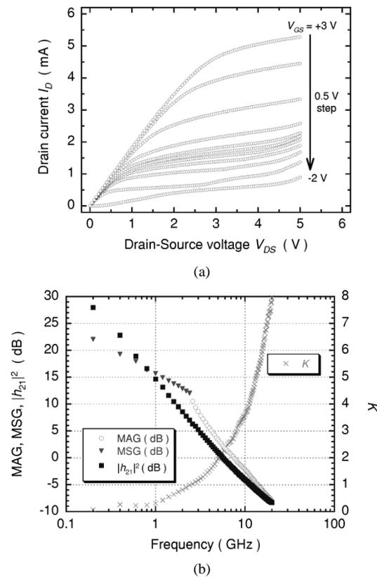
Fig. 11. Measured  $I_D$ - $V_D$  characteristic and the RF characteristics of the GaAs MISFET. The UV and ozone time is 240 min, and the gate length and the gate width are  $1 \mu\text{m}$  and  $80 \mu\text{m}$ , respectively.  $V_{DS} = +4$  V and  $V_{GS} = +1$  V. (a)  $I_D$ - $V_D$  characteristic. (b) RF characteristics.
