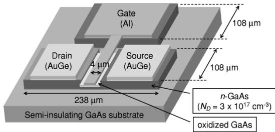
Fig. 5. Structure of the fabricated GaAs MISFET.
