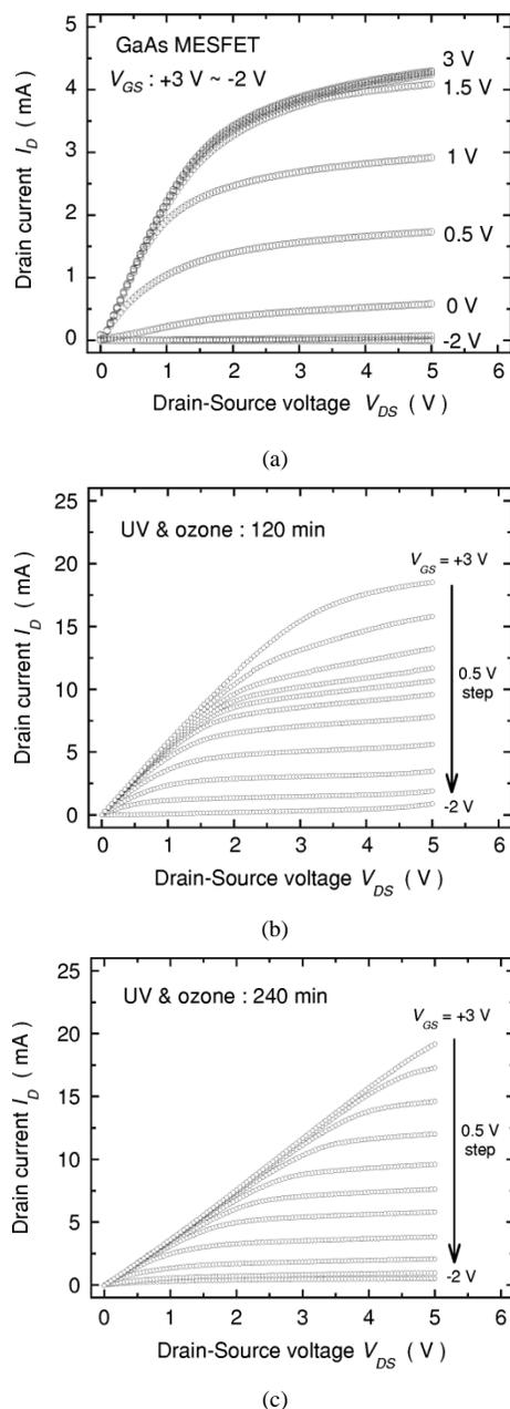
Fig. 8. Drain current-drain voltage ( $I_D$ - $V_D$ ) characteristics for the GaAs MESFET and GaAs MISFET with the UV and ozone times of 120 min and 240 min. The thickness of the oxide layers estimated by the TEM image are 3 nm and 8 nm, respectively. (a) GaAs MESFET. (b) UV and ozone time: 120 min. (c) UV and ozone time: 240 min.
