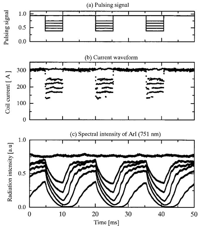
Fig. 10. (a) Spectroscopically measured temporal pulsing signal, (b) modulated current waveform peaks, and (c) radiation intensity of atomic argon at 10 mm below the end coil for Ar-H<sub>2</sub> plasma.
