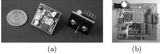
**Figure 4. Developed communication unit(a) and power supply unit(b).**
