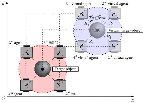
Fig. 2. An example of  $n = 4$  virtual agents enclosing virtual target object.
