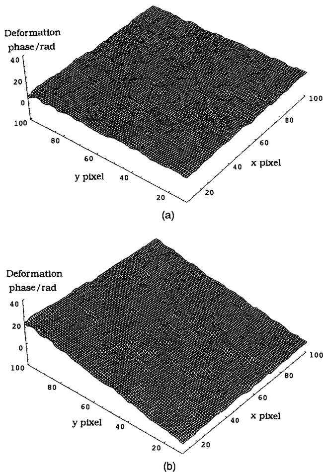
Fig. 9. Whole-field images of the deformation phase where a local area of  $5 \times 5$  pixels and a median filter ( $5 \times 5$ ) were used. (a) From the capturing start  $t_0$  to  $t_{20}$  (20th-frame capturing moment); (b) from the capturing start  $t_0$  to  $t_{200}$ .
