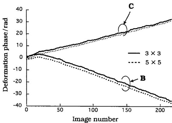
Fig. 8. Time dependencies of deformation phases about points B and C in Fig. 1: solid curves, dependence obtained by using a local area of  $3 \times 3$  pixels; broken curves, that of  $5 \times 5$  pixels.
