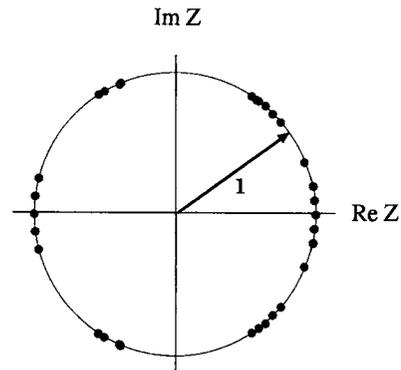
Fig. 3. Complex plane plotting of  $\exp[i\delta_{kl}(\mathbf{r})]$  in a local area ( $3 \times 3$  pixels) where  $\delta_{kl}(\mathbf{r})$  is given by Eq. (3). The number of points is 36 and some overlap.
