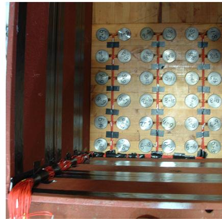
Photo 2 Load cells at the bottom of tank
