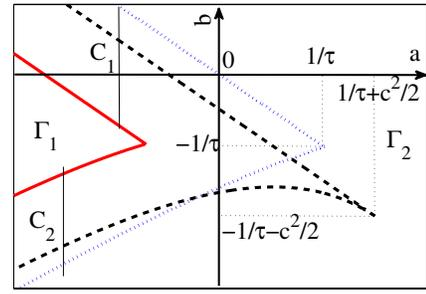
Fig. 2. D-Subdivision for (20) with different  $c$ . Two regions  $\Gamma_1$  and  $\Gamma_2$  show the stable and unstable parameters region for the system (10) respectively.  $C_1$  and  $C_2$  are the boundaries of stable for  $\omega = 0$  and  $\omega \in (0, \pi/\tau)$ .
