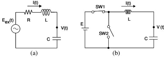
Fig. 2. (a) The general LCR circuit with external voltage  $E_{ex}(t)$ . (b) Step down converter. A switch is composed of nMOS and pMOS transistors.
