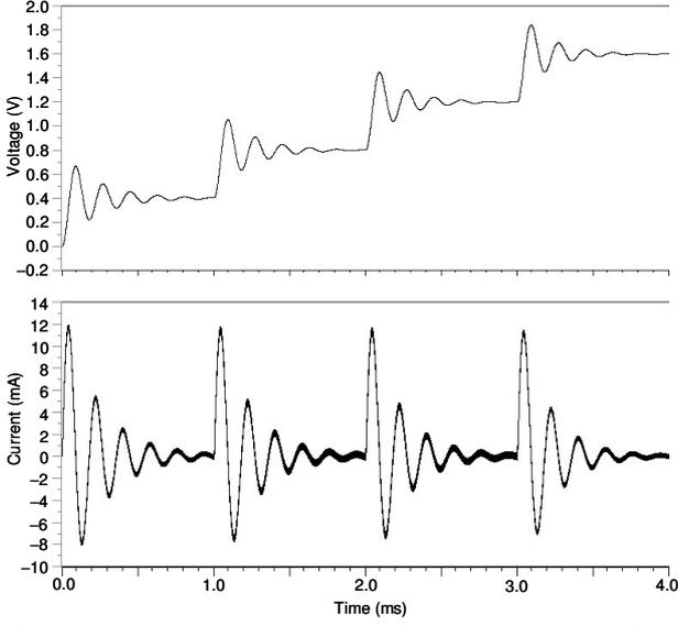
Fig. 5.  $V$  and  $I$  of step down converter when  $L=800\ \mu\text{H}$  and  $C=1\ \mu\text{F}$ .
