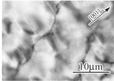
Fig. 2 TEM image of  $\gamma''$  precipitates in the Cu-Ni-Be-Zr specimen aged at 450°C for 2 h after 50% cold-rolling.
