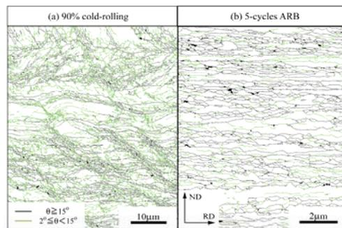
Fig. 1 EBSD boundary maps of the Cu-1.2wt%Ni-0.2wt%Be-0.1wt%Zr specimens, (a) cold-rolled to a 90% reduction and (b) ARB-processed by 5 cycles. In the boundary maps, dotted lines represent the low-angle boundaries having misorientation  $\theta$  of  $2^\circ < \theta < 15^\circ$ , while solid lines indicate the high-angle boundaries with  $\theta > 15^\circ$ .
