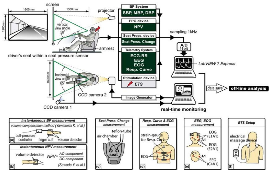
Figure 1 Outline of experimental setup for physiological measurements during simulated monotonous driving. See text for explanation.
