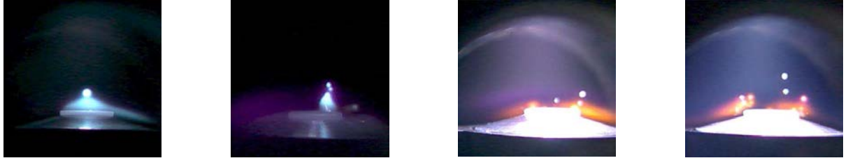
Fig. 5. High-speed video camera captures of thermal plasma irradiated on PA66 specimens with different N_2/O_2 gas mixture ratio.
