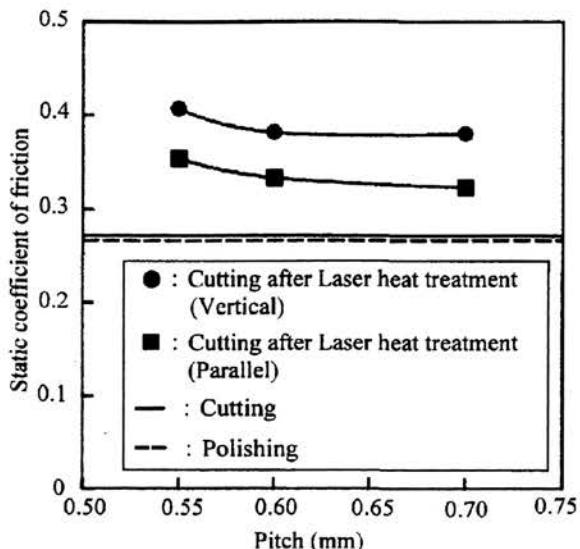
Fig. 6 Influence of Laser pitch on the static coefficient of friction
