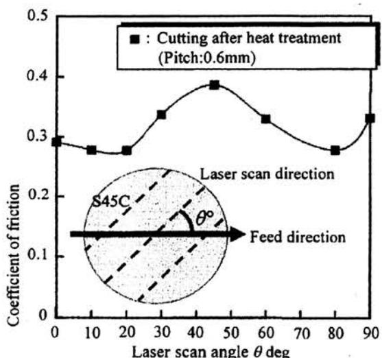
Fig. 8 Influence of Laser scan angle on the static coefficient of friction
