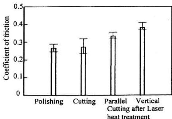
Fig. 5 Influence of finishing process on the static coefficient of friction
