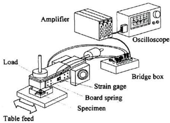
Fig.3 Experimental setup for friction test
