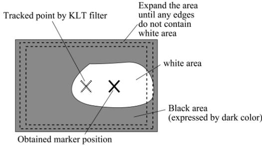
Fig. 7. Estimated marker position based on the tracked point by KLT filter
