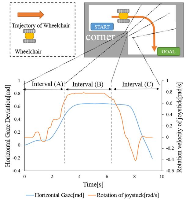
Figure 1. Deviation of gaze angle during wheelchair movement
