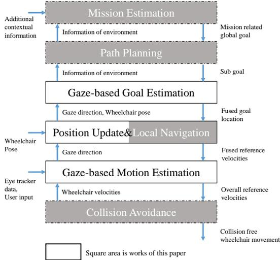
Figure 3. Structure of recursive nested behavior-based control
