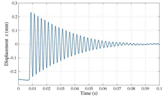
Fig. 6. Displacement at free vibration ( $fr = 392$  Hz).
