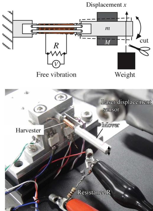
Fig. 4. Experimental setup.
