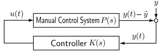
Fig. 2. Closed-loop system of the linearized system  $P(s)$  around the unknown operating point  $\tilde{y}$  in the manual control system and the proposed operator-support controller  $K(s)$ .
