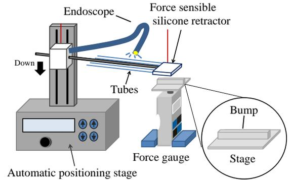
Figure 9. Schematic view of the experimental setup
