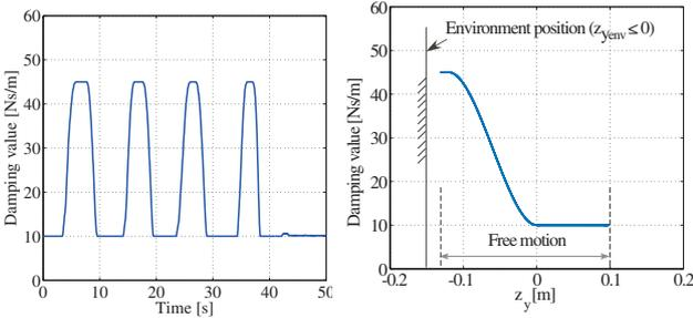
Fig. 7 Varying damping values in free space (Case 1).
