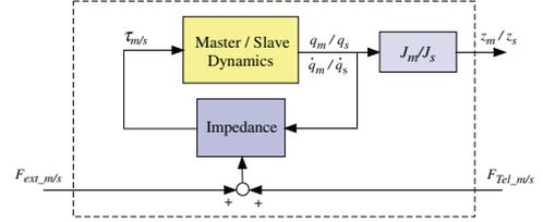
Fig. 2 The master and slave robot dynamics with impedance controller.
