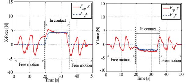
Fig. 9 Force data in contact with environment (Case 2).
