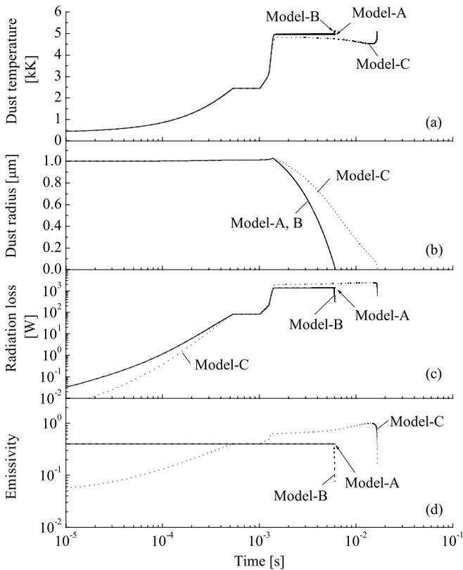
FIG. 3. Temporal evolution of (a) temperature, (b) radius, (c) radiation loss, and (d) the emissivity of the tungsten dust particle in the uniform plasma with parameters:  $T_e=T_i=10$  eV,  $T_a=3$  eV,  $n_e=n_i=n_a=2 \times 10^{13}$  cm $^{-3}$ . Initial dust radius is 1.0  $\mu$ m.
