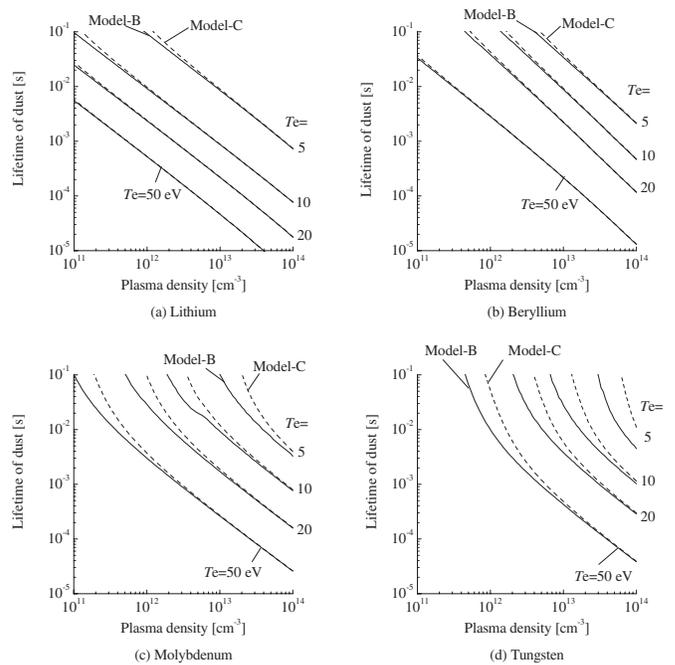
FIG. 4. Lifetime of dust particles displayed for different materials as functions of plasma density and temperature. Plasma parameters are:  $T_i=T_e$ ,  $T_a=0.3T_i$ ,  $n_e=n_i=n_a$ . Initial dust radius is 1.0  $\mu$ m.
