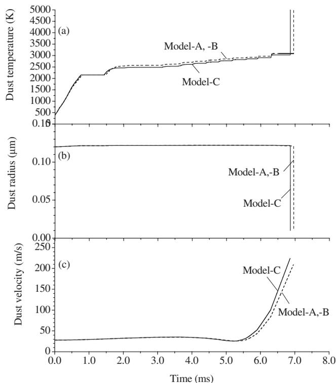
FIG. 7. Time variation in (a) dust temperature, (b) dust radius, and (c) dust velocity in the Alcator C-Mod tokamak corresponding to Fig. 6(b).
