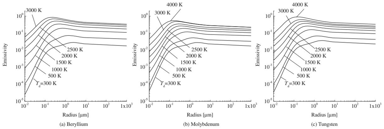
FIG. 1. Emissivity of metallic dust particles as function of dust radius for different dust temperatures as calculated by Mie theory. (a) Beryllium, (b) molybdenum, and (c) tungsten.
