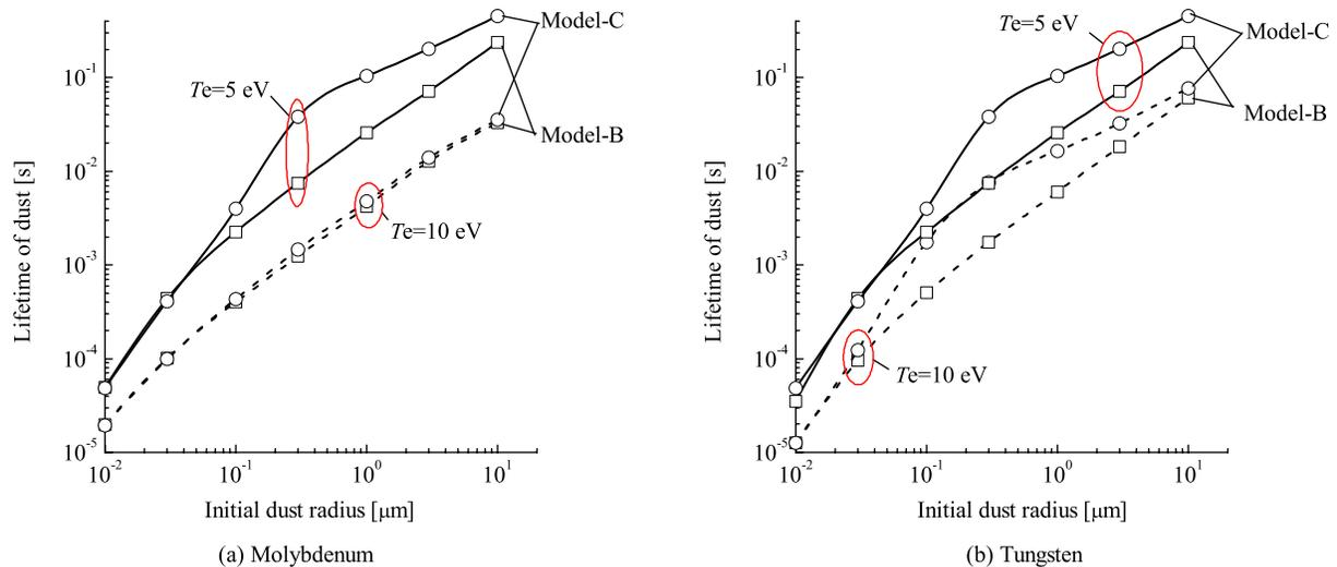
FIG. 5. (Color online) Lifetime of molybdenum and tungsten dust particles as a function of initial dust radius in two types of plasmas: solid curve indicates results with  $T_i=T_e=10$  eV and  $T_a=3$  eV; dotted curve is with  $T_i=T_e=5$  eV and  $T_a=1.5$  eV. For any cases, plasma density is fixed at  $2 \times 10^{13}$  cm $^{-3}$ . (a) Molybdenum dust. (b) Tungsten dust.
