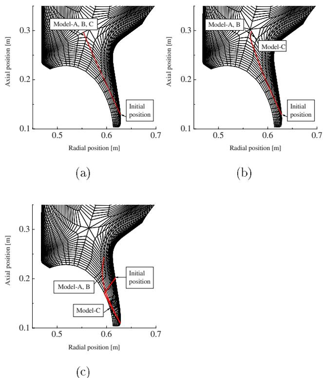
FIG. 6. (Color online) Examples of trajectories of molybdenum dust particle in the edge plasma of the Alcator C-Mod tokamak. (a) Initial radius:  $1.0 \mu\text{m}$ ; initial velocity:  $10 \text{ m/s}$ . (b) Initial radius:  $0.12 \mu\text{m}$ , initial velocity:  $28 \text{ m/s}$ . (c) Initial radius:  $1.0 \mu\text{m}$ ; initial velocity:  $1.0 \text{ m/s}$ .
