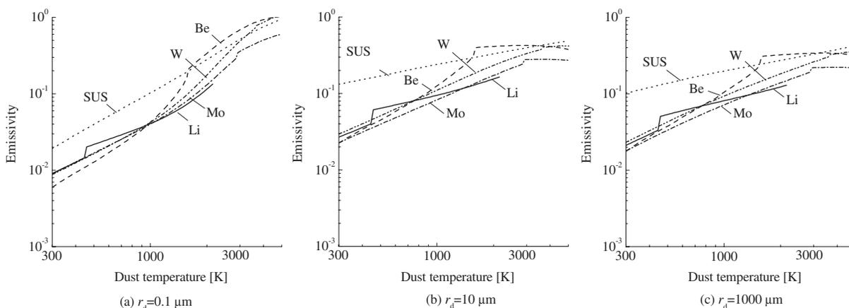
FIG. 2. Emissivity of different metallic dust particles calculated by Mie theory. (a) Dust radius  $r_d=0.1 \mu\text{m}$ , (b)  $r_d=10 \mu\text{m}$ , (c)  $r_d=1000 \mu\text{m}$ .
