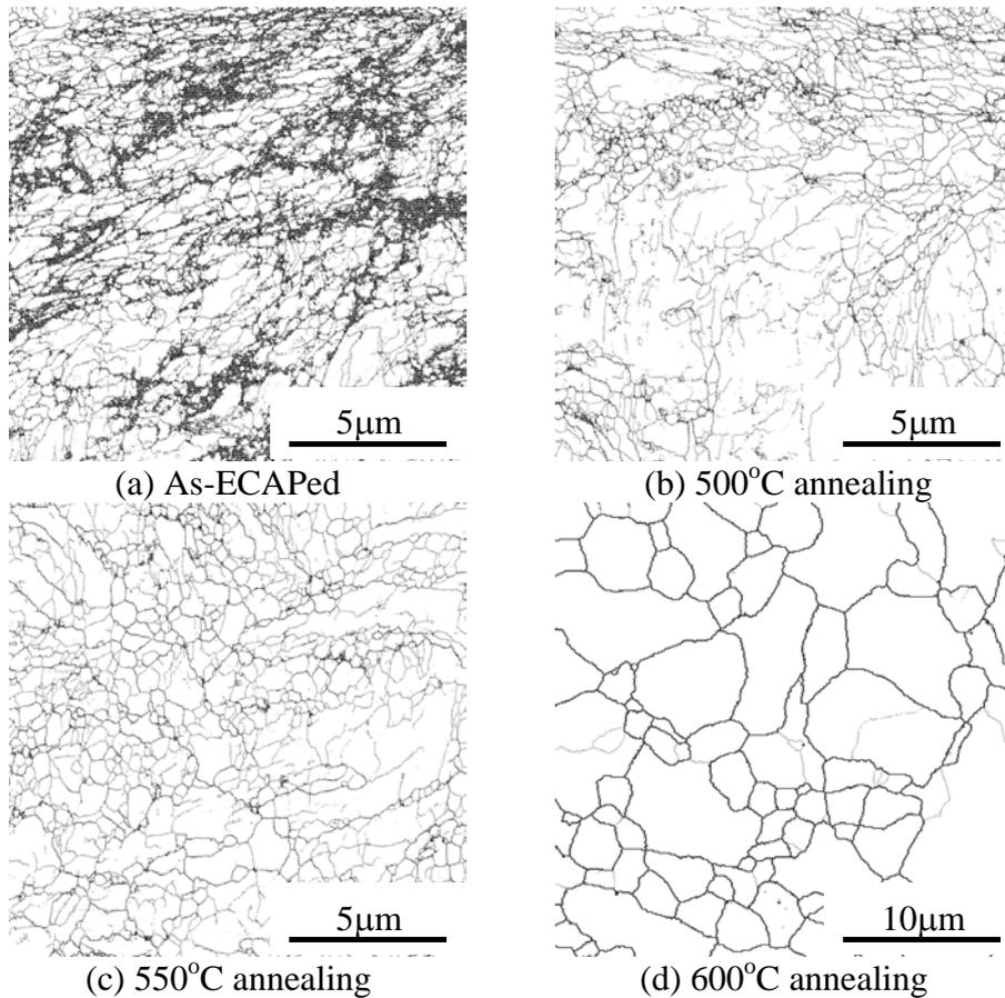
Figure 2. Grain boundary maps of specimens.
