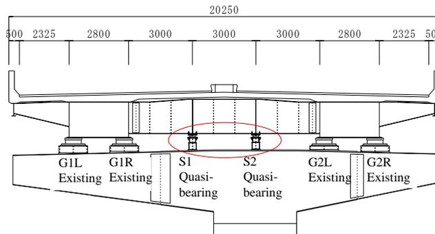
**Figure 3. Position of the Quasi-bearings**
