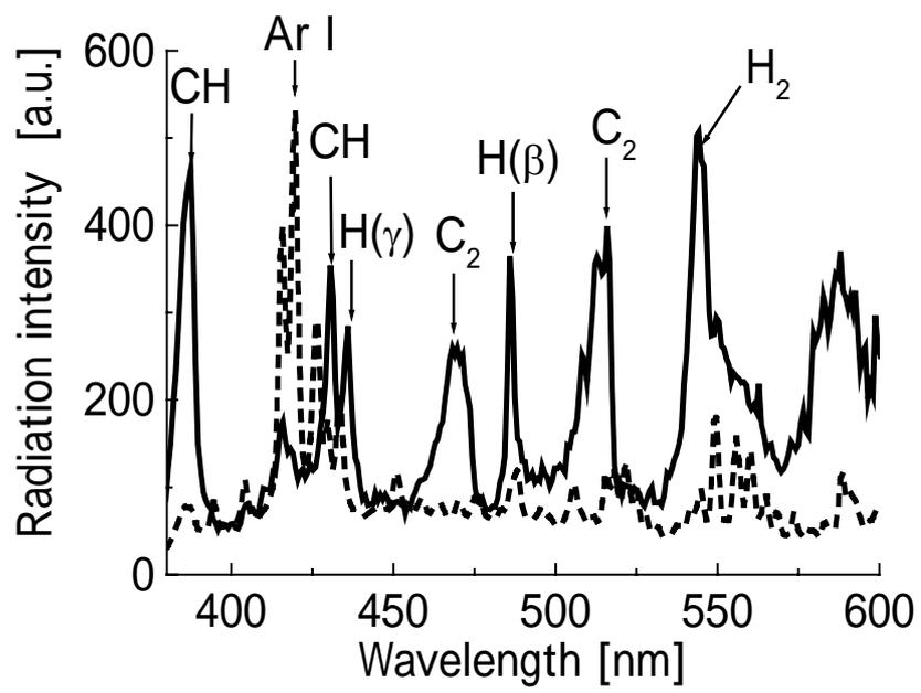
Fig. 3 Radiation spectra from the plasma at 5 mm above graphite target 1 during Ar (dotted line) and Ar/H<sub>2</sub> (solid line) plasma irradiation.
