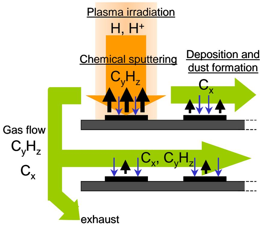
Fig. 7 Schematic illustration of erosion and dust formation in the present experiments
