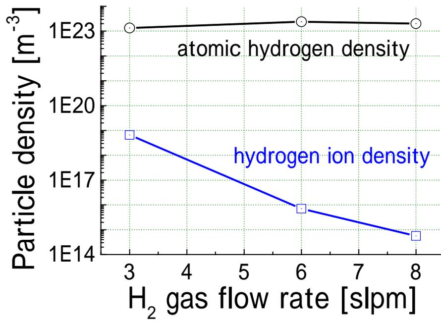
Fig. 2 Atomic hydrogen and hydrogen ion density as a function of the H<sub>2</sub> gas flow rate obtained by fluid simulation.
