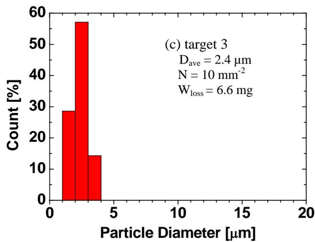
Fig. 6 Size distribution of dust particle on the target 1-3
