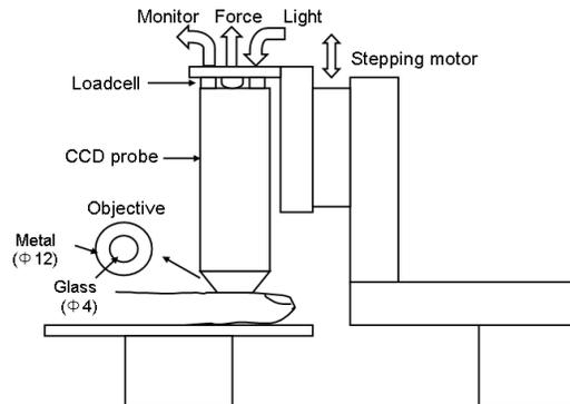
Fig.1 The diagrammatic representation of the system assembly. The capillaroscopy is composed of a CCD video-probe and a contact-type objective lens with a coaxial epi-illumination. The CCD probe was attached to a one-way movable actuator with a force transducer to visualize the dynamic responses of the dermal capillary flow being compressed at the skin surface.
