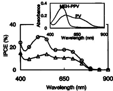
FIG. 3. Photocurrent action spectra of the PV/MEH-PPV *p-n* heterojunction solar cells under an illumination of a normalized  $15 \mu\text{W cm}^{-2}$  monochromatic light. ○ represents the ITO/ In/PV/penetration-treated MEH-PPV/PEDOT/ Au cell and △ represents the ITO/ In/PV/penetration-treated MEH-PPV/ Au cell. The inset shows the absorption spectra of the PV and MEH-PPV.
