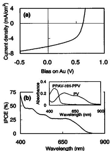
FIG. 5. Photocurrent–voltage characteristic (a) under illumination of a simulated solar light (AM1.5) with  $100 \text{ mW cm}^{-2}$ , and photocurrent action spectra (b) under illumination of a normalized  $15 \mu\text{W cm}^{-2}$  monochromatic light for the ITO/ In/PV/penetration-treated PPAV-HH-PPV/ PEDOT:PSS/Au *p-n* heterojunction solar cells. The inset shows the absorption spectra of the PV and PPAV-HH-PPV.
