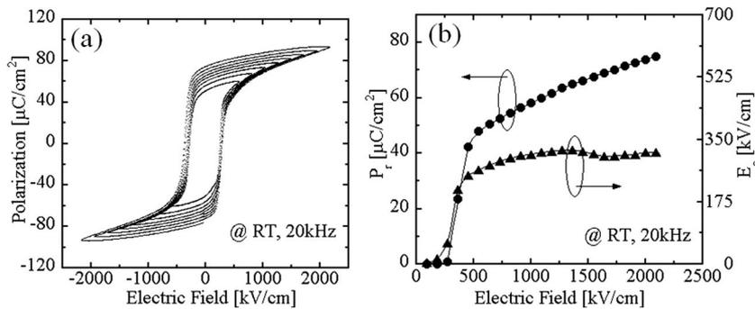
FIG. 3. Ferroelectric properties of BFMT film capacitor measured at RT with measurement frequency of 20 kHz. (a)  $P$ - $E$  hysteresis loops as a function of electric field. (b) Electric field dependences of remanent polarization and coercive field.
