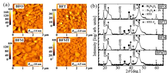
FIG. 1. (Color online) (a) AFM images and (b) XRD patterns for fabricated films grown on Pt-coated (100) STO substrate. The root mean square values of surface roughness of films are shown in the inset of AFM images. Symbols in XRD patterns indicate the impurity phases and substrate.
