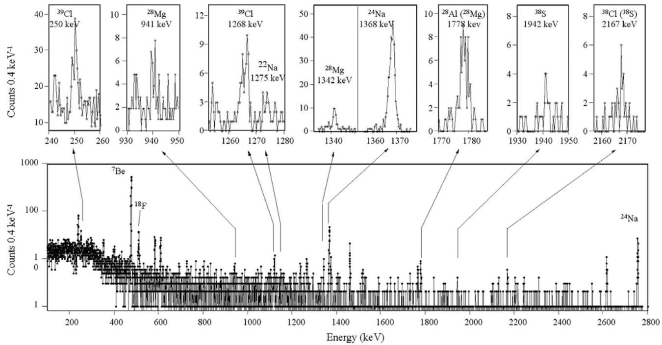
Fig. 1 Gamma ray spectrum of rain sample measured by ultra low-background Ge detector.
