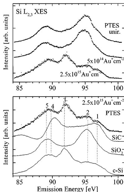
FIG. 5. Silicon  $L_{II,III}$  XES of irradiated PTES films (upper panel) and comparison of spectra of irradiated PTES films and reference compounds (lower panel).
