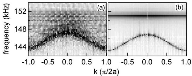
FIG. 4. Simulated production, locking, and decay of ILMs in  $k$  space. Time-space Fourier transform of the displacement for the 500 period time windows identified in Fig. 3(a): They are at (i) 2000 and (ii) 7000 periods, respectively. Frame (a) shows the time development at the end of the chirp and (b), at the end of the locked state. For reference the linear dispersion curve of the upper band is shown (dotted).
