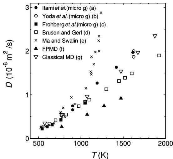
FIG. 15. The self-diffusion coefficient,  $D$ , of liquid Sn as a function of temperature,  $T$ ; microgravity experiments: (a) Itami *et al.*, (Ref. 11), (b) Yoda *et al.* (Ref. 12), and (c) Frohberg *et al.* (Refs. 9 and 10); experiments on the ground: (d) Bruson and Gerl (Ref. 62) and (e) Ma and Swalin (Ref. 61); molecular dynamics (MD): (f) the present first-principle MD (FPMD), and (g) the present classical MD.
