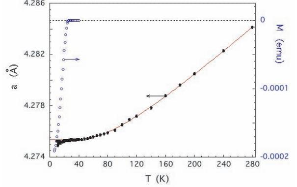
Figure 2: Plots of lattice parameter  $a$  (solid circles: left-hand scale) and magnetization (open circles: right-hand scale) of  $\text{Ba}_{0.6}\text{K}_{0.4}\text{BiO}_3$  versus temperature. The red solid line is the least-squares fit obtained using a simple Einstein model above  $T_c$  and its extension below  $T_c$ .
