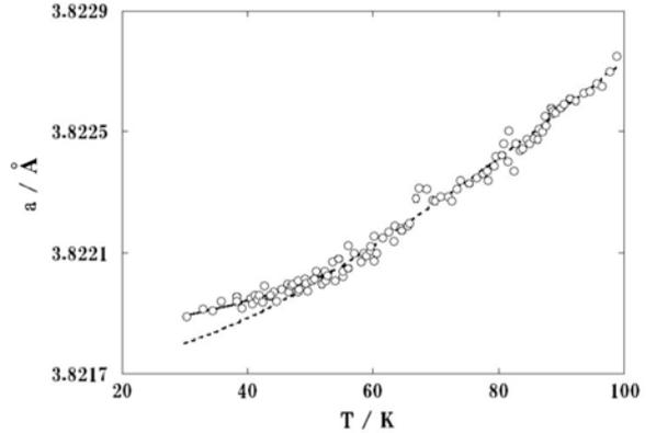
Figure 4: Comparison between the observed lattice parameter  $a$  (open circles) and the calculated one (solid line in superconducting phase) of orthorhombic  $\text{YBa}_2\text{Cu}_3\text{O}_{6.5}$  ( $T_c = 55$  K). The observed  $a$  values were obtained from Ref. 1. The broken line is the least-squares fit obtained using a simple Einstein model above  $T_c$  and its extension below  $T_c$  (see text).
