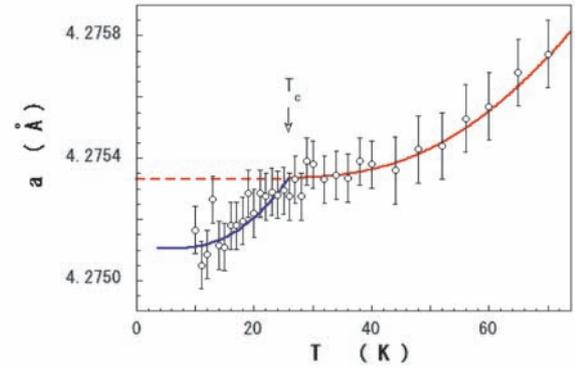
Figure 3: Comparison of the lattice parameter  $a$  (open circles) and the square of the BCS gap (blue solid line below  $T_c$ ) of  $\text{Ba}_{0.6}\text{K}_{0.4}\text{BiO}_3$ . The red solid line and the broken line are the least-squares fits obtained using a simple Einstein model above  $T_c$  and its extension below  $T_c$ , respectively. (see text). The square of the BCS gap is reversed, whose origin is taken at  $a(T_c)$  obtained by fitting.
